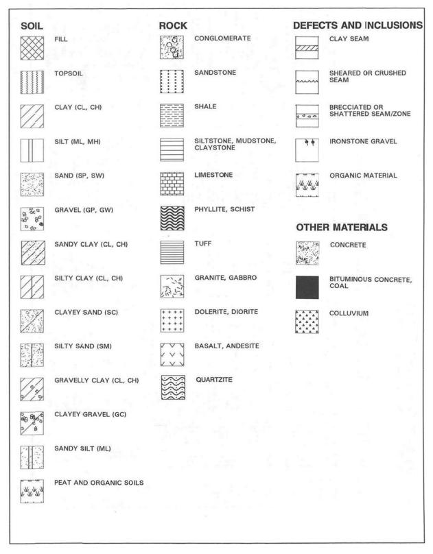
The following information is intended to assist in the interpretation of terms and symbols used in geotechnical borehole logs, test pit logs and reports issued by or for the JC Geotechnics Pty Ltd. More detailed information relating to specific test methods is available in the relevant Australian Standards AS1726-2017.
